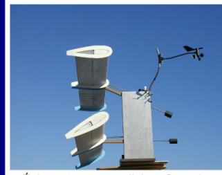
Éolo prototype, parallel configuration, operating in air.
